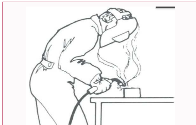
Figure 3: Rising plume of fume and gases from weld spot.
