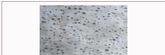
Figure 2a: Microstructure of the Ductile.
