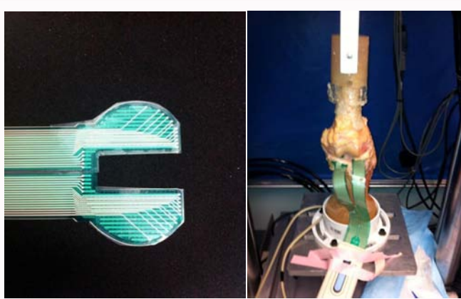
Figure 1: Tekscan 410-N knee sensor, with proper placement in the cadaveric knee.
