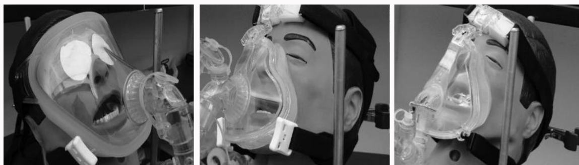
Figure 2: Three interfaces tested from left to right, full face mask, oronasal mask, and Performa track mask.
