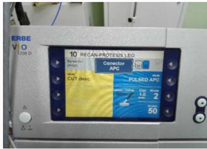
Figure A: ERBE 200D equipment was used, with flow 1.0, effect 2, 50 watts, 4300 Vp, APC mode, recan-prosthesis program, circumferential and frontal probe interchangeably.
