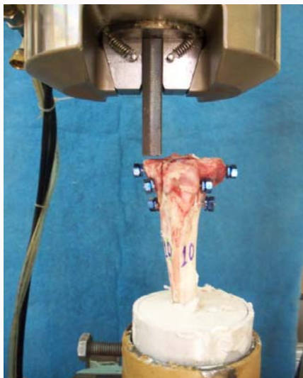
Figure 3: The EFECE system was attached to the jaws of the material testing system servo hydraulic testing machine and increasing compression force was applied to these systems.
