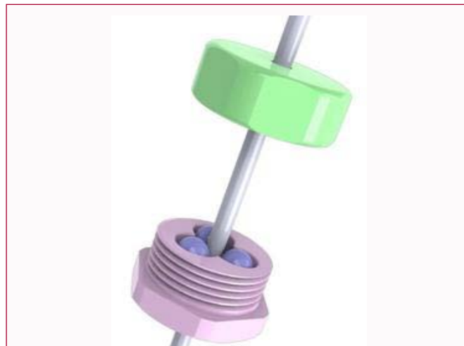
Figure 1: The EFECE implant contains two pieces that are attached to each other with threads. The top piece functions as a cap. The second piece contains 3 gloves for the insertion of 3 balls. These balls are 2.5 mm radius and magnetic active. The angle of the cone shaped gloves to the K-wire axis is 7°. There is a hole for insertion of a 1.2 mm K-wire in each piece.
