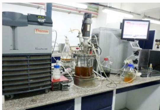
Figure 2: A Biofo 310 fermentor; 7 L (New Brunswick Scientific, Edison, NJ, USA).
