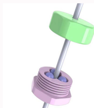
Figure 1: The prototype of this EFECE implant contains two pieces that catch each other with threads. The top piece functions as a cap. The second piece contains 3 gloves for the insertion of 3 metal balls. These balls are with 2.5 mm radius and magnetically active. The cone-shaped gloves angle to the k-wire axis is 7 degree. There is a hole for the insertion of 1.2 mm k-wire at each piece.
