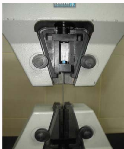
Figure 3: EFECE implant and k-wire system attached to the Lloyd Instruments LR 50K Universal Materials Testing Machine with the help of jaws and increasing distraction force and cycling loading applied to these systems.
