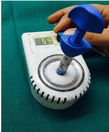
Figure 1: Digital wax melter with wax replaced by common salt used as a composite warmer.
