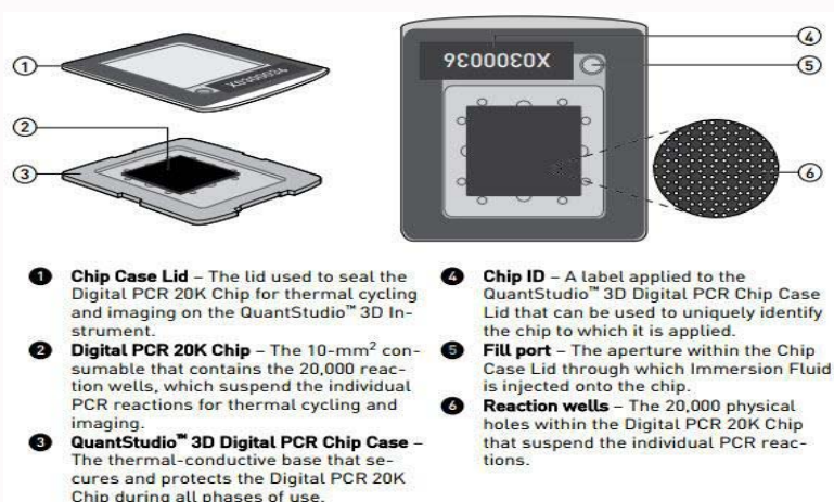
Figure 2: Diagram illustrating QuantStudio™ 3D Digital PCR System Chip; ChipCase Lid (1); Digital PCR 20K 10 mm 2 nanofluidic v2 chip (2), which contains 20,000 reaction wells; QuantStudio™ 3D Digital PCR Chip Case (3); Chip ID (4); Fill port (5); and Reaction wells, the 20,000 physical holes that suspend individual PCR reactions.
