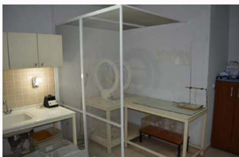
Figure 3: Helmholtz Coils placed in the Faraday cage.
