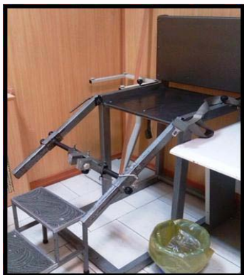
Figure 1: The designed chair to measure the knee extensor torque.
