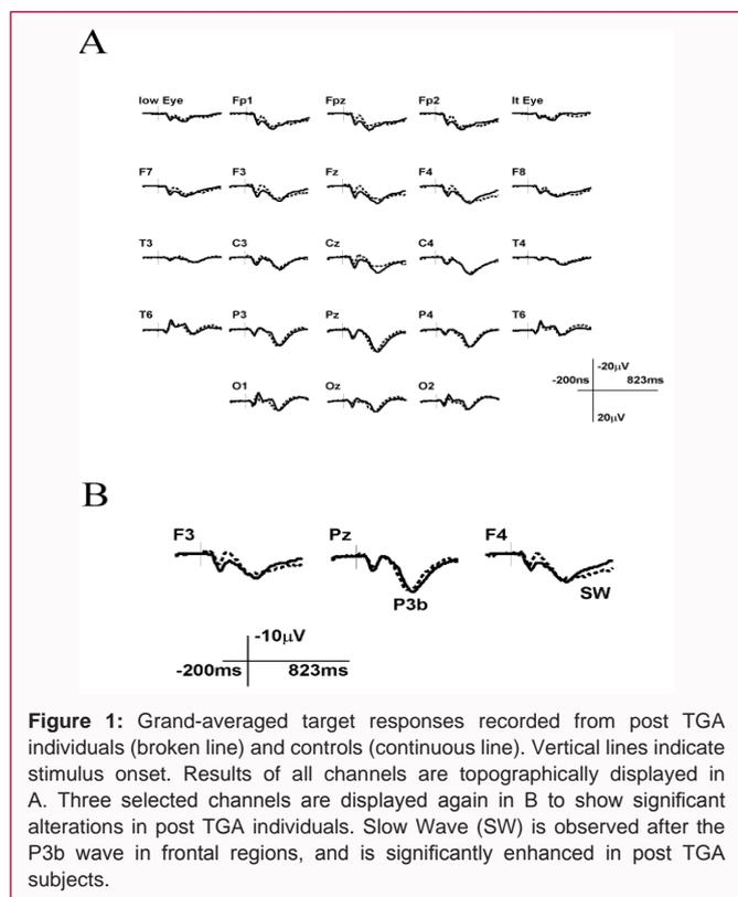
**Figure 1:** Grand-averaged target responses recorded from post TGA individuals (broken line) and controls (continuous line). Vertical lines indicate stimulus onset. Results of all channels are topographically displayed in A. Three selected channels are displayed again in B to show significant alterations in post TGA individuals. Slow Wave (SW) is observed after the P3b wave in frontal regions, and is significantly enhanced in post TGA subjects.
