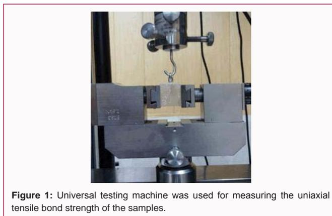
**Figure 1:** Universal testing machine was used for measuring the uniaxial tensile bond strength of the samples.
