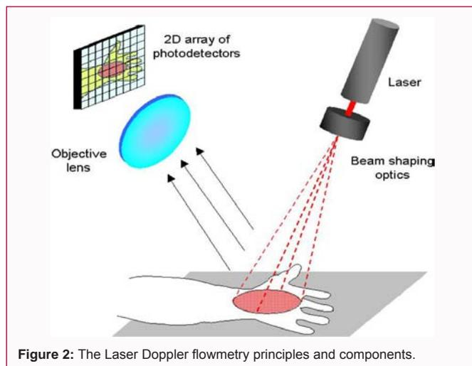
Figure 2: The Laser Doppler flowmetry principles and components.
